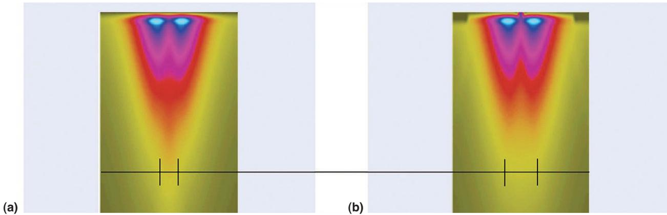
Figure 1. Beam simulation: (a) flat plate; (b) 4.5 in. (11.43 cm) OD pipe.
