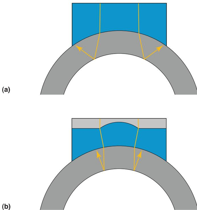
Figure 2. Beam divergence path: (a) a standard wedge; (b) passive-axis focusing wedge.
