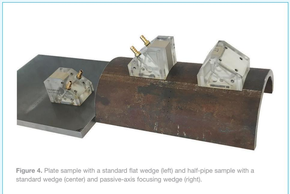
Figure 4. Plate sample with a standard flat wedge (left) and half-pipe sample with a standard wedge (center) and passive-axis focusing wedge (right).
