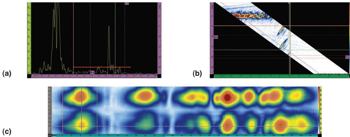
Figure 7. Views of data acquired with a standard wedge on a 4.5 in. (11.43 cm) OD pipe: (a) A-scan; (b) S-scan; (c) C-scan.
