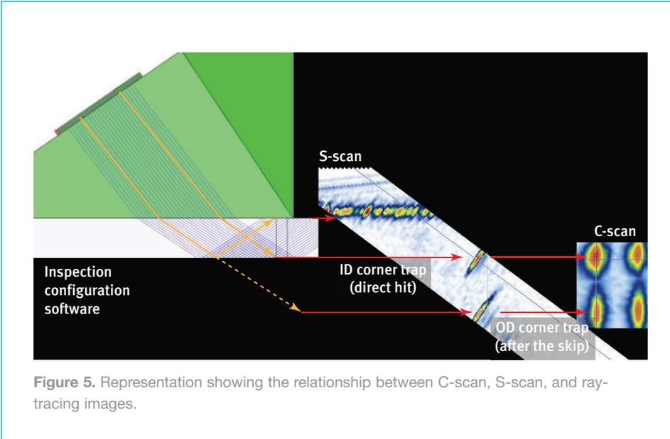
S-scan view (center), the ID corner trap appears higher than the OD corner trap as it arrives earlier in time. On the C-scan view (right), the OD and ID corner traps are represented on top of each other for every through-hole in the scan direction.
