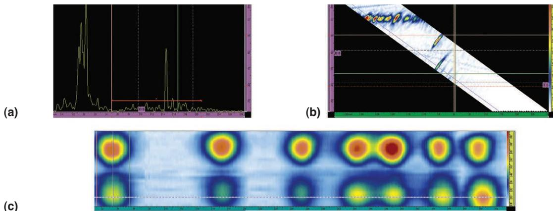
Figure 8. Views of data acquired with a passive-axis focusing wedge on a 4.5 in. (11.43 cm) OD pipe: (a) A-scan; (b) S-scan; (c) C-scan.
