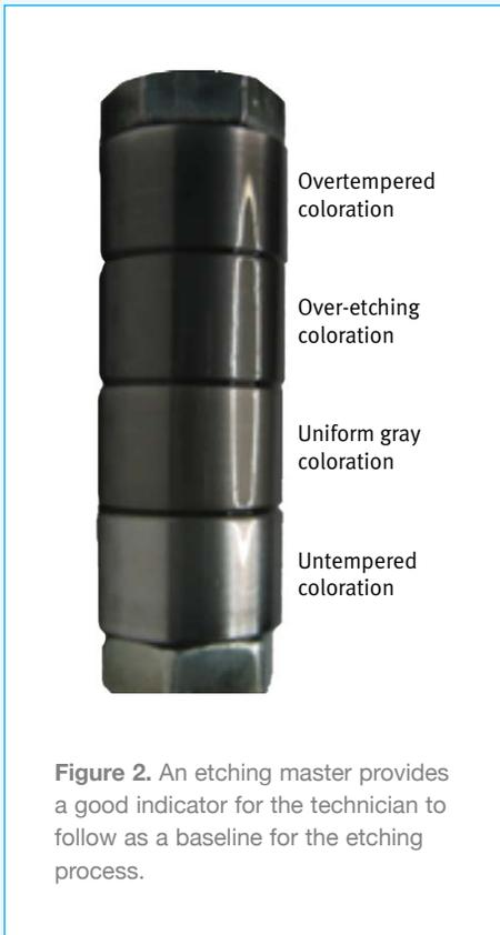
**Figure 2.** An etching master provides a good indicator for the technician to follow as a baseline for the etching process.
