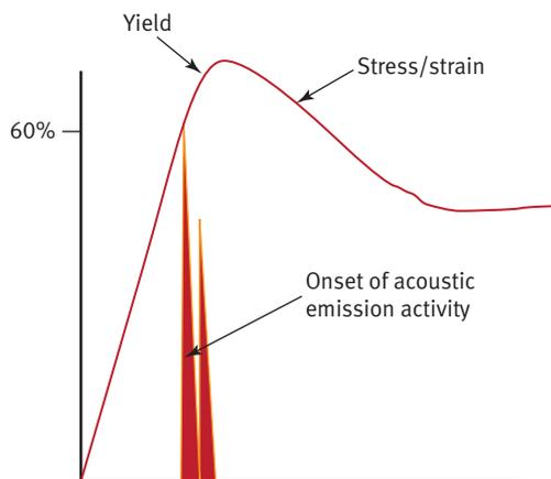
Figure 1. Stress/strain versus acoustic emission activity.
