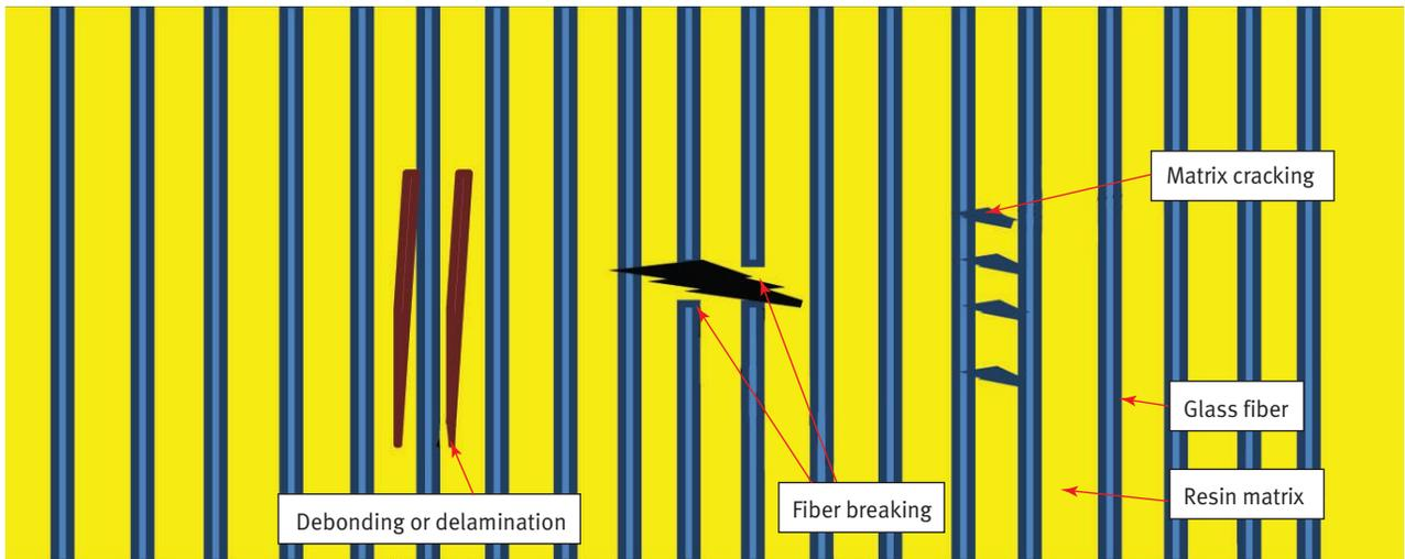
**Figure 10.** Typical discontinuities in fiber-reinforced plastic material.
