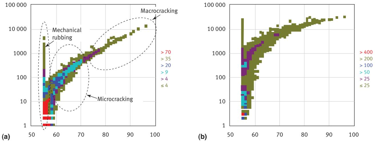
**Figure 9.** Correlation plots of the acoustic emission hit data showing mechanical rubbing, microcracking, and macrocracking: (a) energy versus amplitude versus hits; (b) duration versus amplitude versus hits.
