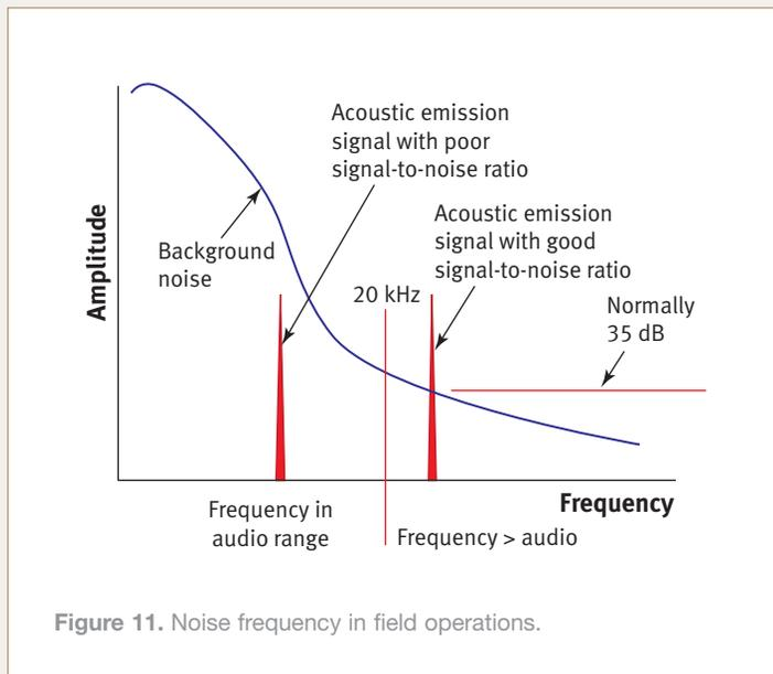
sources. The choice of the bandwidth used in the data collection should consider the effect of the frequency on the attenuation, thus reducing the effective sensor-to-source distance. The higher the frequency of the bandwidth that is used, the greater the reduction on the sensor-to-source distance.
