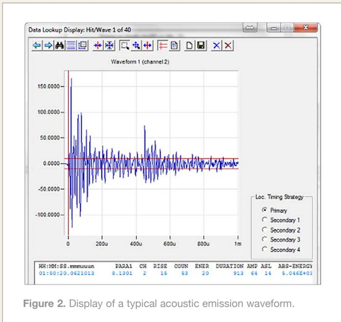
Figure 2. Display of a typical acoustic emission waveform.
