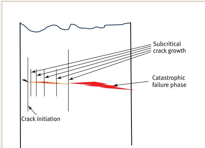
**Figure 4.** Basic crack behavior: crack initiation, subcritical crack growth, and catastrophic failure.
