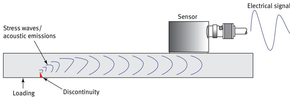
Figure 1. Acoustic emission stress waves.
