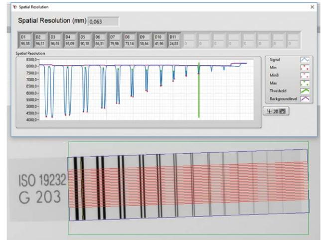
Figure 2. Spatial resolution measurement with double-wire IQI.
