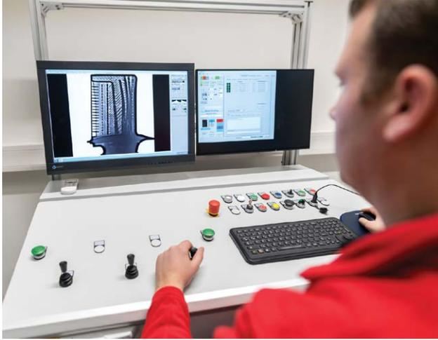
Figure 1. Digital inspection of a turbine blade.
