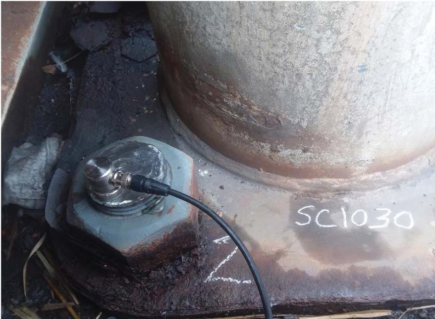
Figure 5. Transducer over a reject indication.
