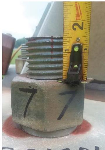
Figure 6. An example of a cracked anchor bolt: (a) top view; (b) side view.
