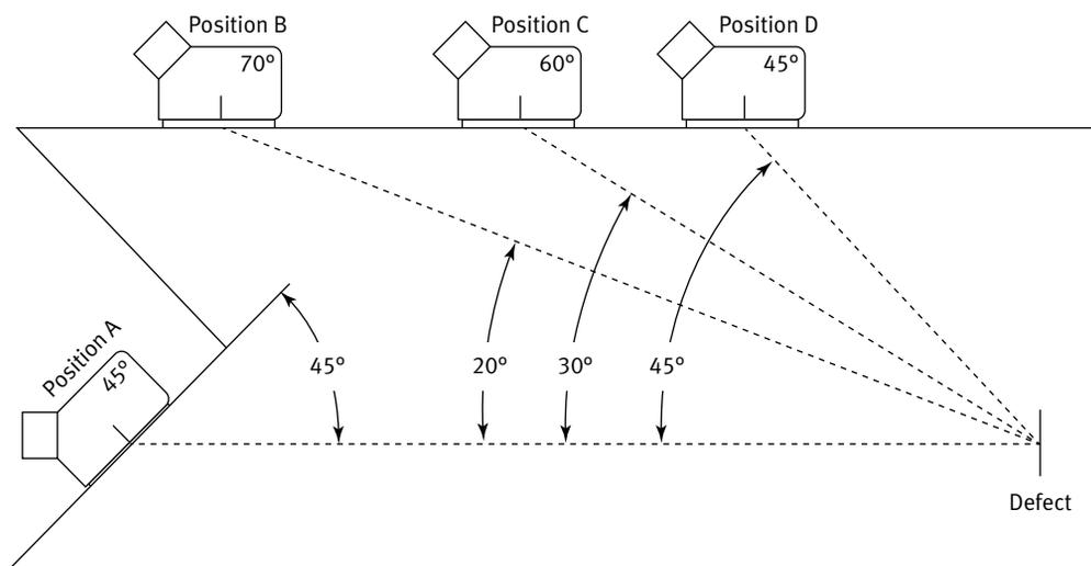
Figure 1. Basis of the AWS indication rating technique.
