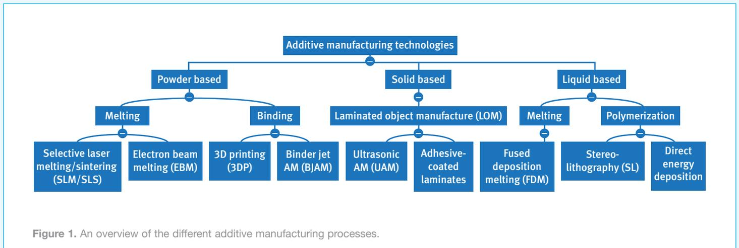
Figure 1. An overview of the different additive manufacturing processes.
