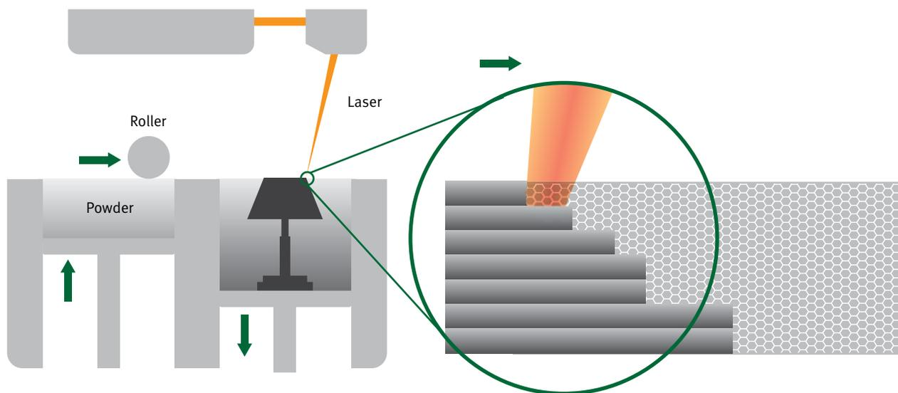
Figure 2. How the selective laser sintering process works.
