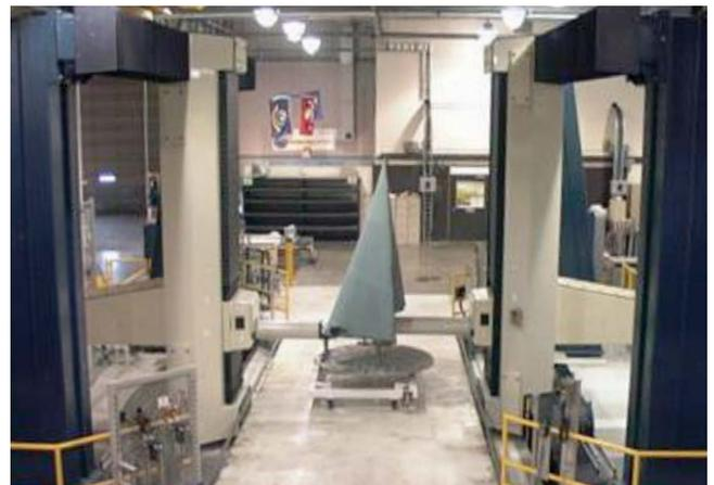
Figure 5. Multiple-axis squirter UT system for inspection of composite structures with complex contours.
