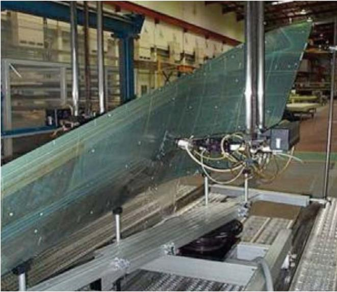
Figure 3. Gantry scanner inspection of a large aircraft component.
