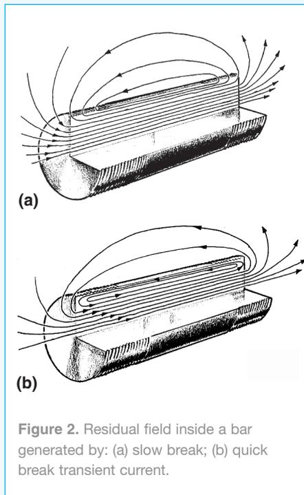
**Figure 2.** Residual field inside a bar generated by: (a) slow break; (b) quick break transient current.
