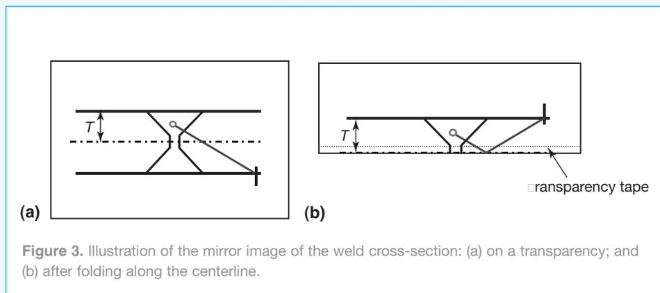
Figure 3. Illustration of the mirror image of the weld cross-section: (a) on a transparency; and (b) after folding along the centerline.
