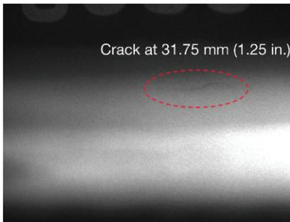
Figure 5. Radiography of a detected crack with its depth found by performing ultrasonic testing.
