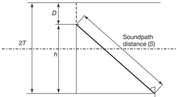
Figure 4. Simple geometry used to calculate the discontinuity depth from the mirror image.
