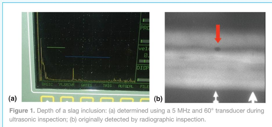
**Figure 1.** Depth of a slag inclusion: (a) determined using a 5 MHz and 60° transducer during ultrasonic inspection; (b) originally detected by radiographic inspection.
