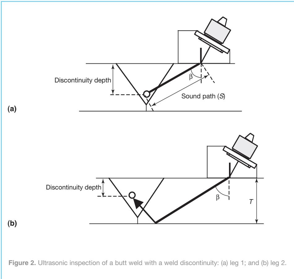
Figure 2. Ultrasonic inspection of a butt weld with a weld discontinuity: (a) leg 1; and (b) leg 2.
