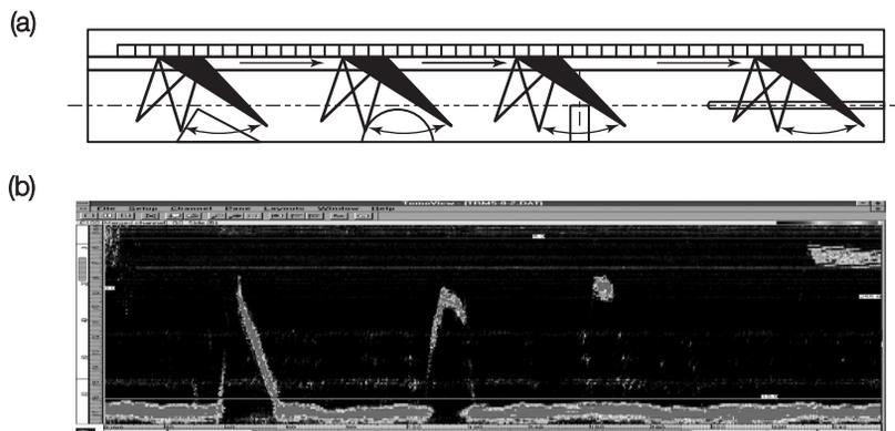
Figure 6. Phased array imaging patterns: (a) scanning pattern using sectorial and linear scanning; (b) image using all data merged together.
