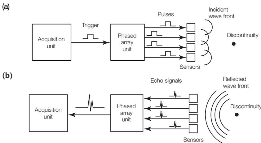
Figure 2. Beam: (a) emitting; (b) receiving.
