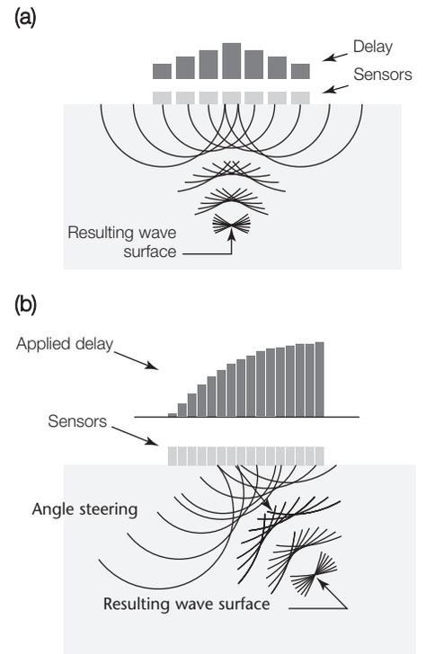
Figure 3. Schematic time delays (histograms): (a) focused normal beam; (b) focused transverse wave.
