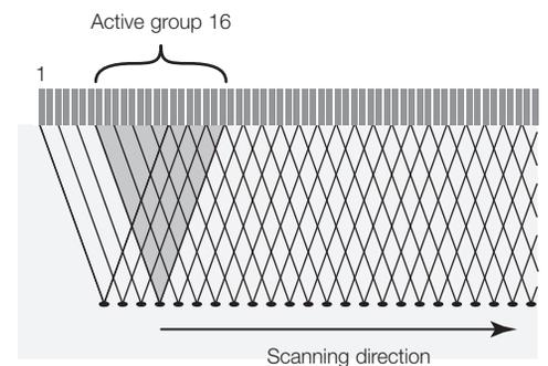
Figure 4. Electronic scanning.
