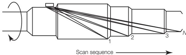
Figure 5. Sectorial scanning on turbine rotor for sequence of  $N$  scans.
