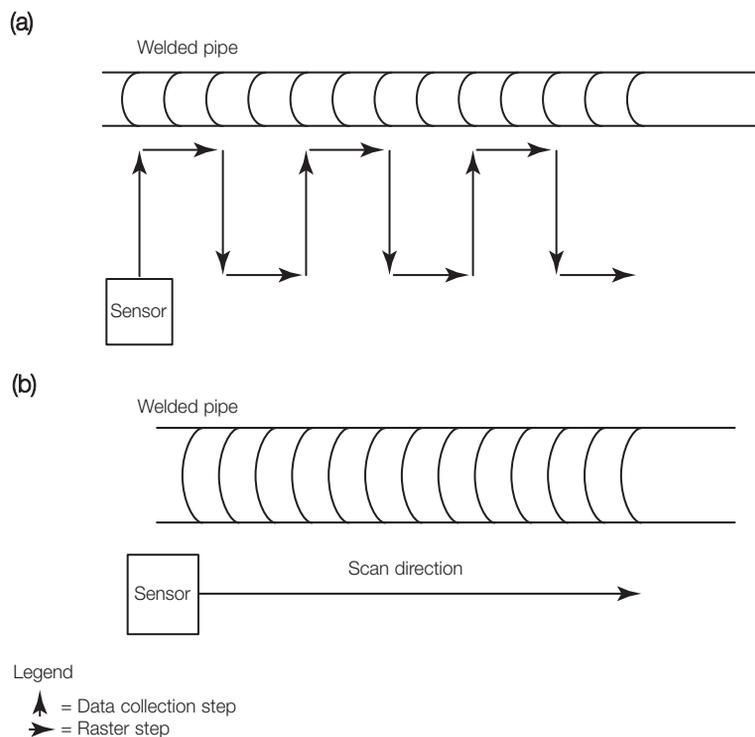
Figure 7. Scanning: (a) conventional raster; (b) linear.
