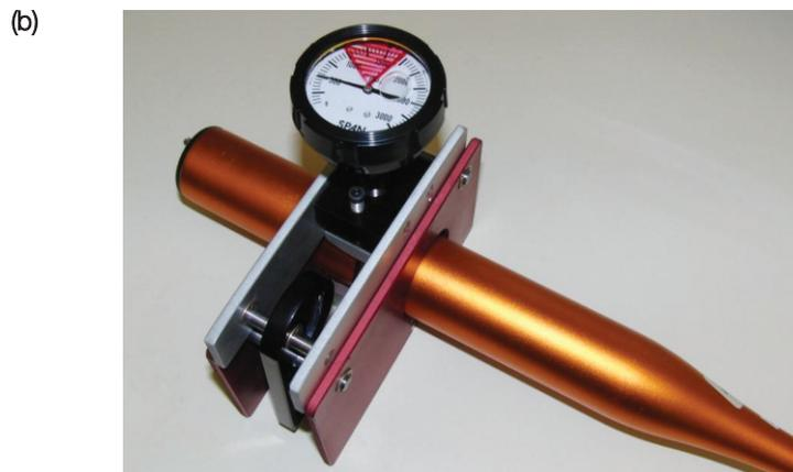
Figure 3. Barrel compression testers measure barrel stiffness of hollow composite or aluminum softball bats: (a) setup for laboratory testing and (b) portable device.
