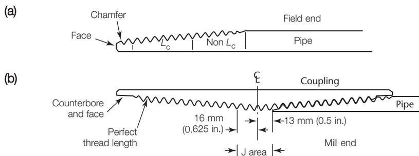
Figure 3. Round thread areas: (a) pin, (b) coupling.
