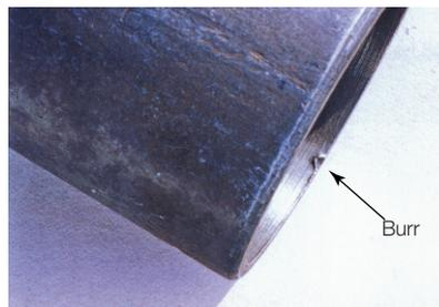
Figure 4. Burr on end of coupling.
