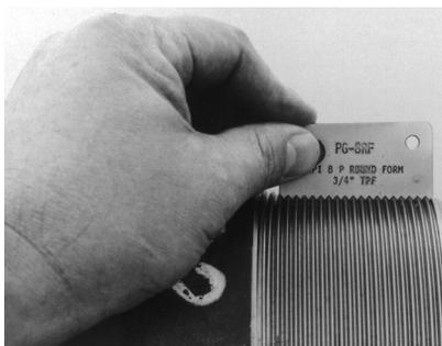
Figure 2. Profile gage on round threads.
