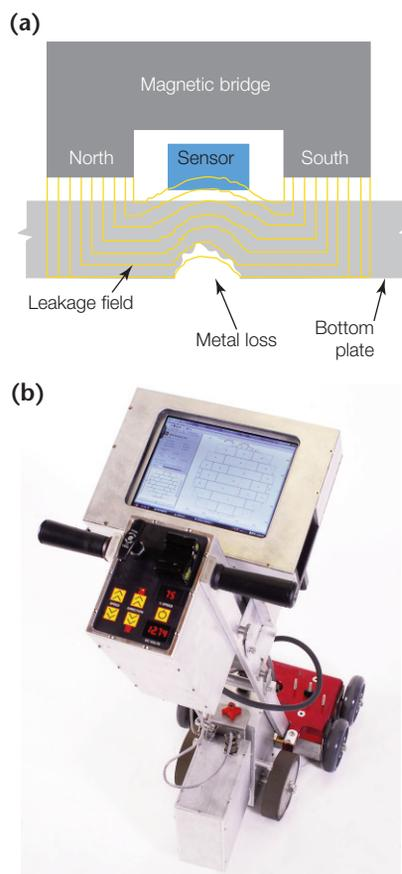
Figure 2. Magnetic flux leakage method: (a) schematic of bridge; (b) tank bottom scanner incorporating magnetic flux leakage test bridge.
