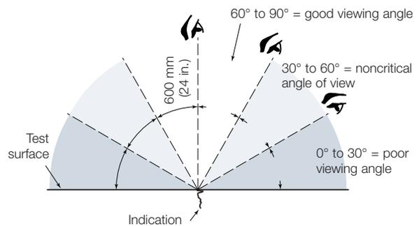
Figure 2. Good and poor angles of view.
