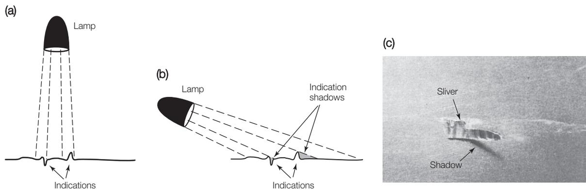
Figure 4. Angle of illumination: (a) no indication shadows; (b) indication shadows (c) photo of sliver with shadow.
