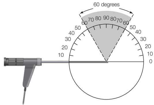
Figure 5. Field of view of rigid borescope.
