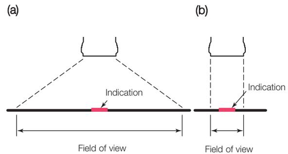
Figure 6. Effect of field of view on magnification at 90 degree angle: (a) with wide field of view, indication is one tenth as wide as image; (b) with zoom, indication is half as wide as image.
