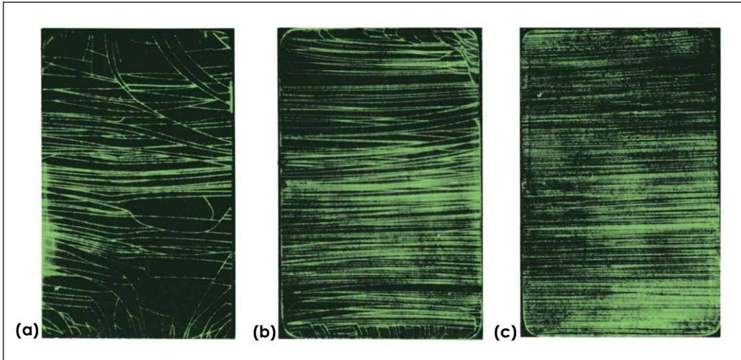
**Figure 3. Fluorescent indications of stress cracks in chrome-plated nickel test panels: (a) coarse cracks; (b) medium cracks; and (c) fine cracks.**
